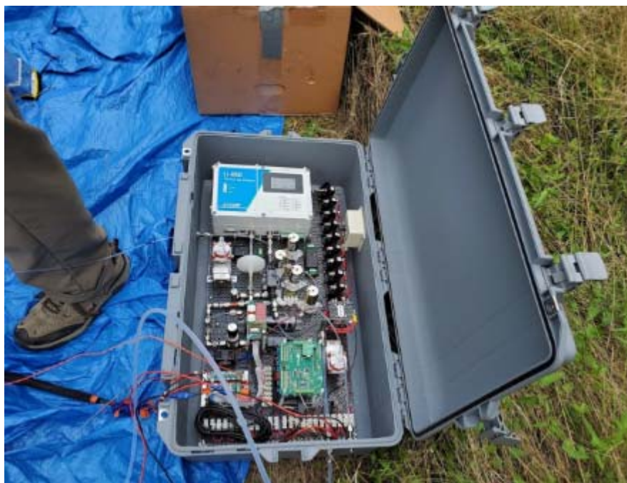
Figure 2-4. Comprehensive terpenoid EF measurement system control, power and CO 2 /H 2 O sensor.
