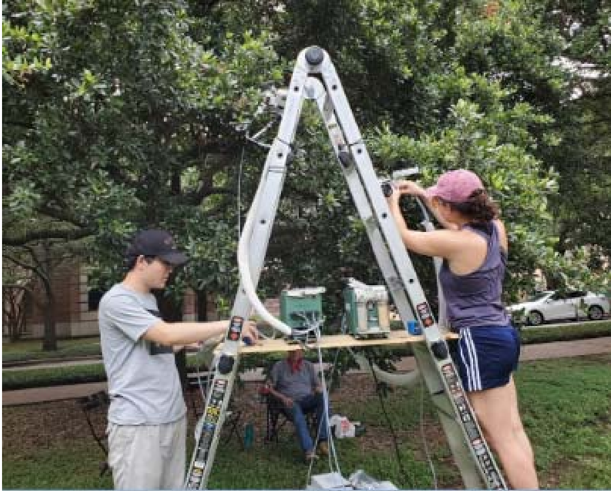
Figure 2-1. Ladder platform deployment of LICOR 6400 systems for isoprene measurements on an oak tree on the Rice University campus.
