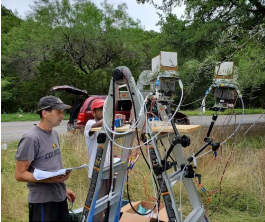
Figure 2-3. Comprehensive terpenoid EF measurement systems enclosing 2 sets of leaves on a mesquite tree near Austin TX.
